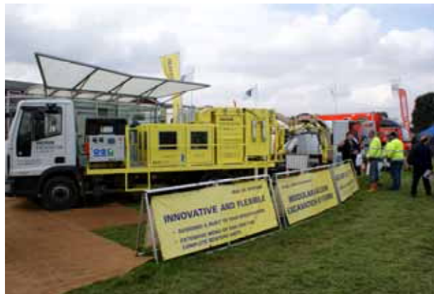
The new Mod Ex 5000C vacuum excavation unit (5000 cfm/chassis mounted) on show at the recent No-Dig Live exhibition, in this instance as a 7.5 tonne Iveco truck-mounted unit with a 4.3 m wheelbase and a 1.2 m 3 spoil tank.
