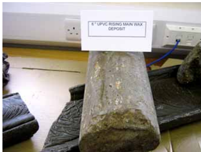
Blocks of solidified wax removed from both the gravity sewer and rising main sections.
